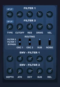
2 FILTERS - LOW PASS, BAND PASS AND HIGH PASS, EACH WITH TWO-POLE OR FOUR-POLE OPTION
