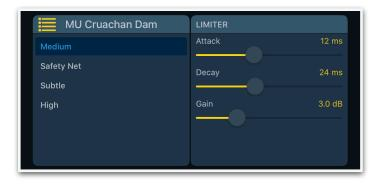
The Cruachan Dam limiter is a simple peak limiter that allows you to create a "mastered" loudness effect, or simply catch high transients with the "safety net" preset. Optimum attack and decay times depend on the nature of the signal being processed, but the defaults are good general-purpose settings.
