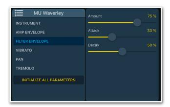
This is the default Waverley view seen here running in GarageBand on iPhone. On iPad, if the host window is large enough, a larger view is displayed showing all parameters. The left pane defaults to a categories selector, in this case, the filter envelope. The right pane shows the parameters and their values for that category. That's it basically! Unselecting a category will expand the right hand view to show a table view of all parameters.
